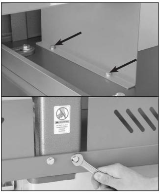
Figure 22. Installing guard with removed bolts.
